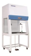
Chemical fume hoods are designed to protect personnel and prevent contaminants from escaping into the laboratory environment. All fume hoods work by drawing air from the room and mixing it with contaminated air in the hood. This air is then drawn up a duct and expelled out of the building. Interference with this airflow can compromise the hood's ability to protect the user. The following chemical fume hood types are approved for use on universities:
